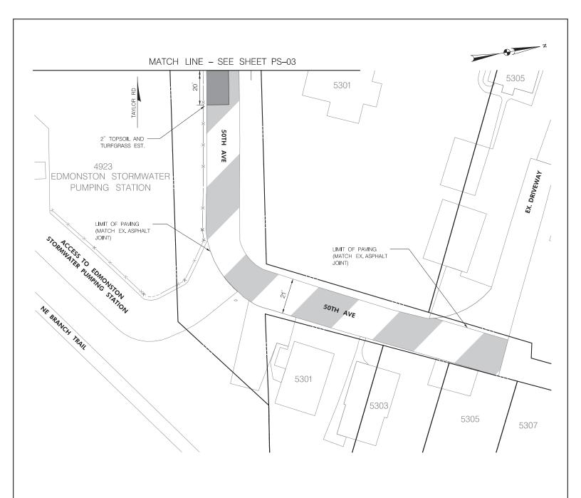
APPROXIMATE SELECTED QUANTITIES ON THIS SHEET DESCRIPTION UNITS QTY MILL EXIST PAVEMENT 2 INCH SY 637 2 INCH HMA SURFACE 9.5MM PG 64-22 TON 75 6 INCH HMA BASE 19.0MM PG 64-22 TON 11 6 INCH GRADED AGGREGATE SUBBASE SY 30 (GASB) COURSE SY 23 TURFGRASS ESTABLISHMENT TOPSOILING - 2 INCH CLASS 2 EXCAVATION SY 23 CY 12
